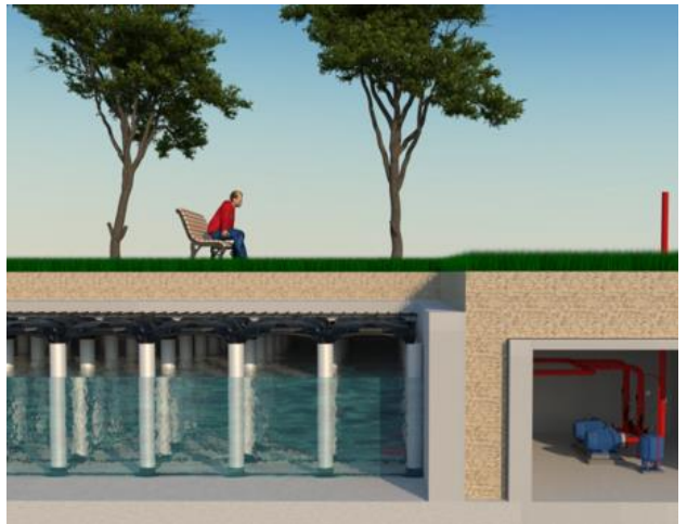
WATER HARVESTING STORAGE / STORMWATER ATTENUATION TANK
